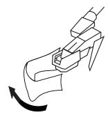
8 Turn the TURNTABLE SUSPENSION SCREW clockwise until it is all the way down.
