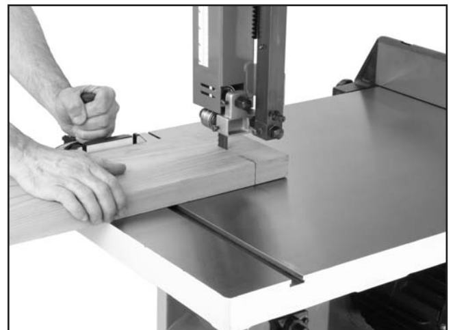
Figure 41. Example of crosscutting operation with miter gauge.
