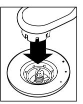
amount of silicon grease to the valve O-ring and reassemble. If the valve is not leaking around its
