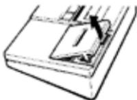
2. Peel off the glued edge of the printing paper included with the unit, and cut it off to about 2 inches with a pair of scissors, and then shape and cut the edge for easy insertion to the printer as shown in the figure.
