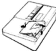
5. When the PRINT/PAPER FEED button is pressed while the results of the measurement are shown on the digital display, these results, together with the date and time of measurement are printed out.
