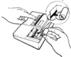
4. Insert the printing paper in the installation section, and then attach the cover back to the main unit in such a way that the edge of the paper protrudes from the cover.
