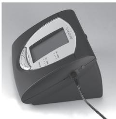
2. To use your 1157 without batteries, use **ONLY** the included AC adapter. Plug the adapter into the unit first, then into the wall outlet.
