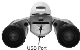
**Note:** You cannot load to a Unix system using the camera's USB port—this port can download only to Windows OS or Mac OS 9.0 or higher.
