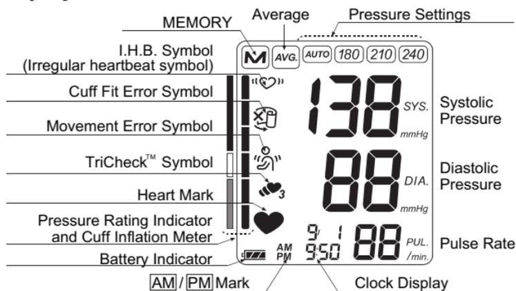
A&D blood pressure monitors are easy to use, accurate and digitally display full measurement readouts. Our technology is based on the "oscillometric method" - a noninvasive blood pressure determination. The term "oscillation" refers to any measure of vibrations caused by the arterial pulse. Our monitor examines the pulsatile pressure generated by the arterial wall as it expands and contracts against the cuff with each heartbeat.
