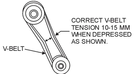
Figure 9. V-Belt Tension
