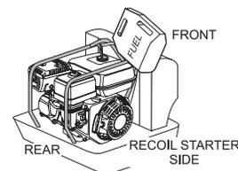
Since spilled fuel could ignite if it comes into contact with hot engine parts, **ALWAYS** pour fuel from the **recoil starter side** of the compactor. Allow engine to **cool!** before refueling. Wipe up any spilled fuel immediately.
