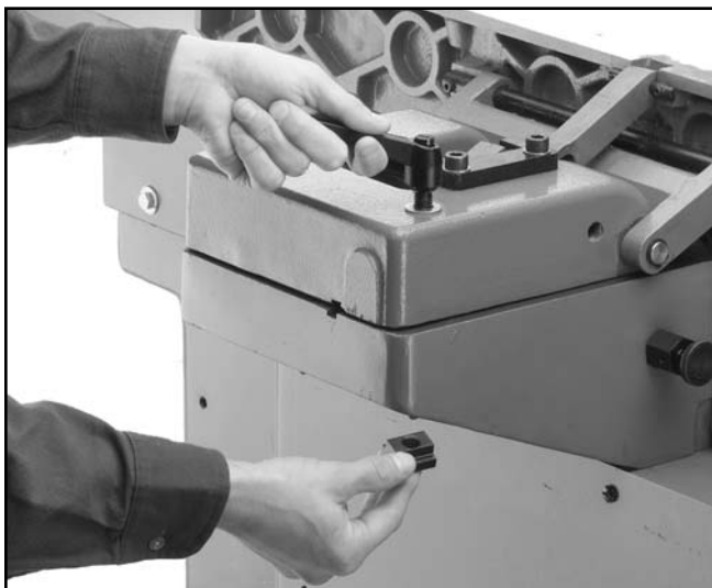
Figure 5. Fence base lock knob attachment.
