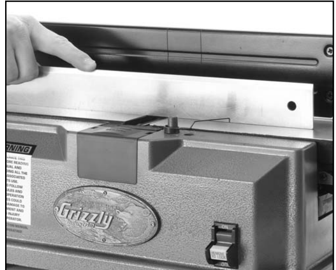
Figure 6. Straightedge across outfeed table.
