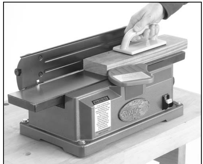
Figure 16. Typical surface planing operation.
