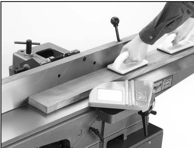
Figure 27. Correct method for surface planing.
