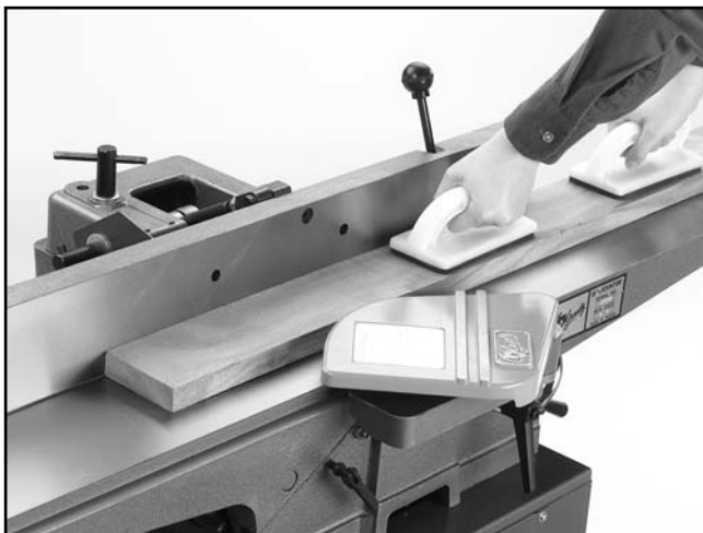
Figure 27. Correct method for surface planing.
