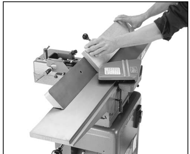
Figure 26. Fence position for bevel jointing.
