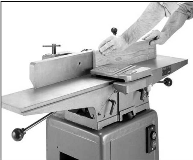
Figure 25. Operator position for edge joining.
