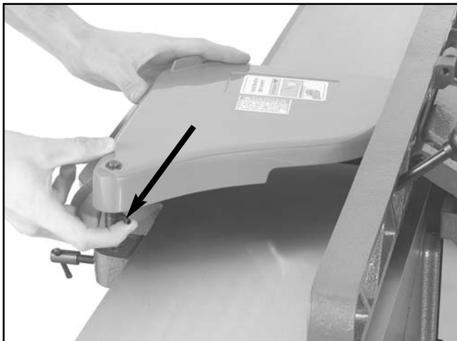
Figure 36. Installing cutterhead guard while holding spring tang.
