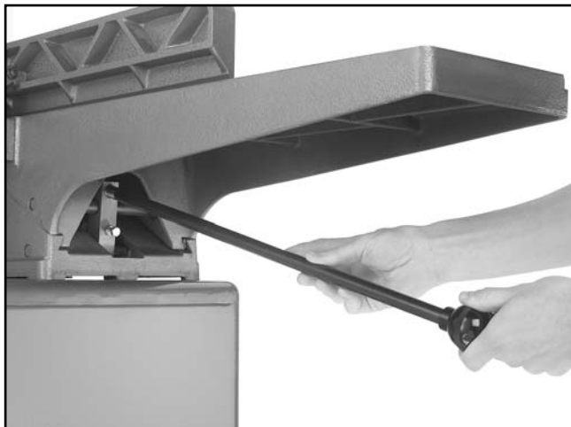
Figure 25. Installing table lever into adjustment block.
