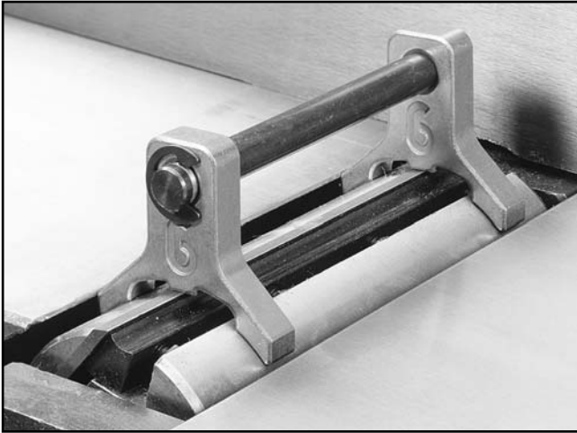
Figure 53. Jig placement on cutterhead.
