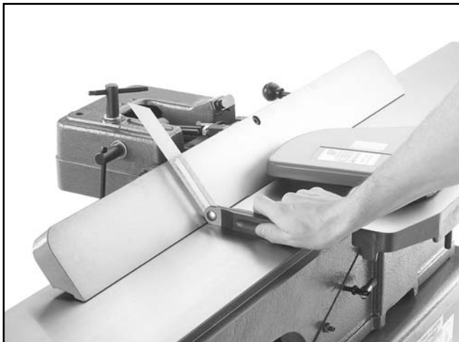
Figure 40. Checking the fence at 45°R with a bevel gauge.
