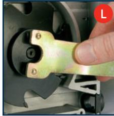
5. Remove the outer blade flange (fig M).
