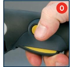
5. The lock-on button allows the operator to keep the biscuit joiner motor running without continuously holding the switch. It is useful when operating the tool for extended periods.
