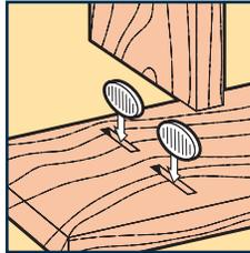
To cut the biscuit slot, the body of the joiner is moved toward the material. By utilising the various features of the tool you can create a wide range of different types of joints.
