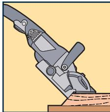
1. Slots for a mitre joint can be cut with the workpiece secured flat on the bench and the fence tilted to the required angle.
