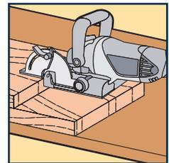
3. Cut the slots into the workpiece that will become the vertical board.
