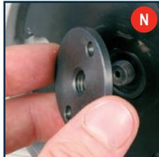
5. Remove the outer blade flange (fig N).
