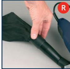
2. The dust bag (14) can be connected to the adaptor (fig R).
