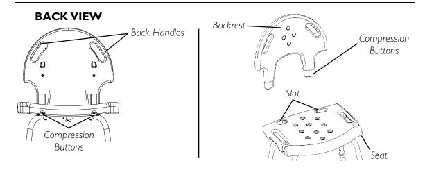
FIGURE 2 - INSTALLING/REMOVING THE BACKREST ON MODELS 9681P AND 9681
