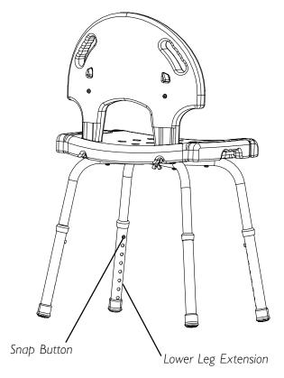
FIGURE 3 - ADJUSTING THE LEG EXTENSIONS
