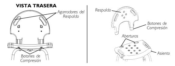
FIGURA 2 - INSTALANDO/REMOVIENDO EL RESPALDO EN LOS MODELOS 9681P Y 9681
