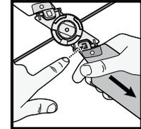
**NOTE:** If you have difficulty removing the blade, press the button on the clip with a pen or other thin object
