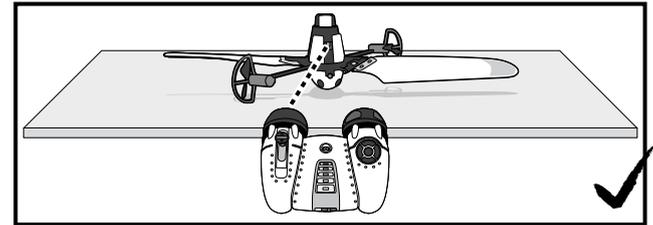
5. On the controller push the throttle slowly to control the height and power, press and hold the direction buttons to direct FlyTech Bladestar left, right, forwards and backwards.
