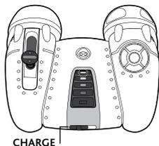
**NOTE:** If the top LED indicator on the controller blinks repeatedly, it indicates that FlyTech Bladestar is already fully charged.
