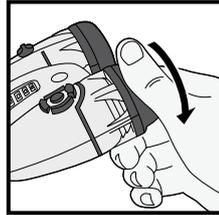
3. Hold FlyTech Bladestar firmly by the core and insert the charger cable into the socket as illustrated. Pay close attention to the orientation of the socket and the connector on the cable.
