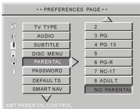
3. Push [RIGHT] to enter the sub-menu in the right of the screen, if you want to change the age control grade to 3, push [DOWN] till the high lighting band move to the item "3PG", the player will indicate you to enter password, if the ex-factory password has never been modified, you can push number buttons "4408" in the remote control.
