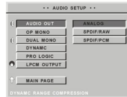
2. Push [RIGHT] to enter the sub-menu in the right screen, push [DOWN] to move the high lighting band to the item "SPDIF/RAW" or "SPDIF/PCM", then push [ENTER].
