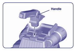
• "Snap" the handle into the top of the jet, as shown.
