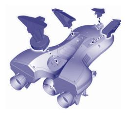
• "Snap" the nose gear, both main landing gear pieces and the handle to the bottom of the shuttle.
