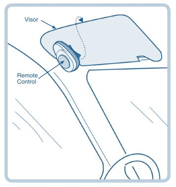
• Attach the remote control clip to the top of the vehicle visor. *Hint:* The remote control does not need to be in direct line with dashboard.
