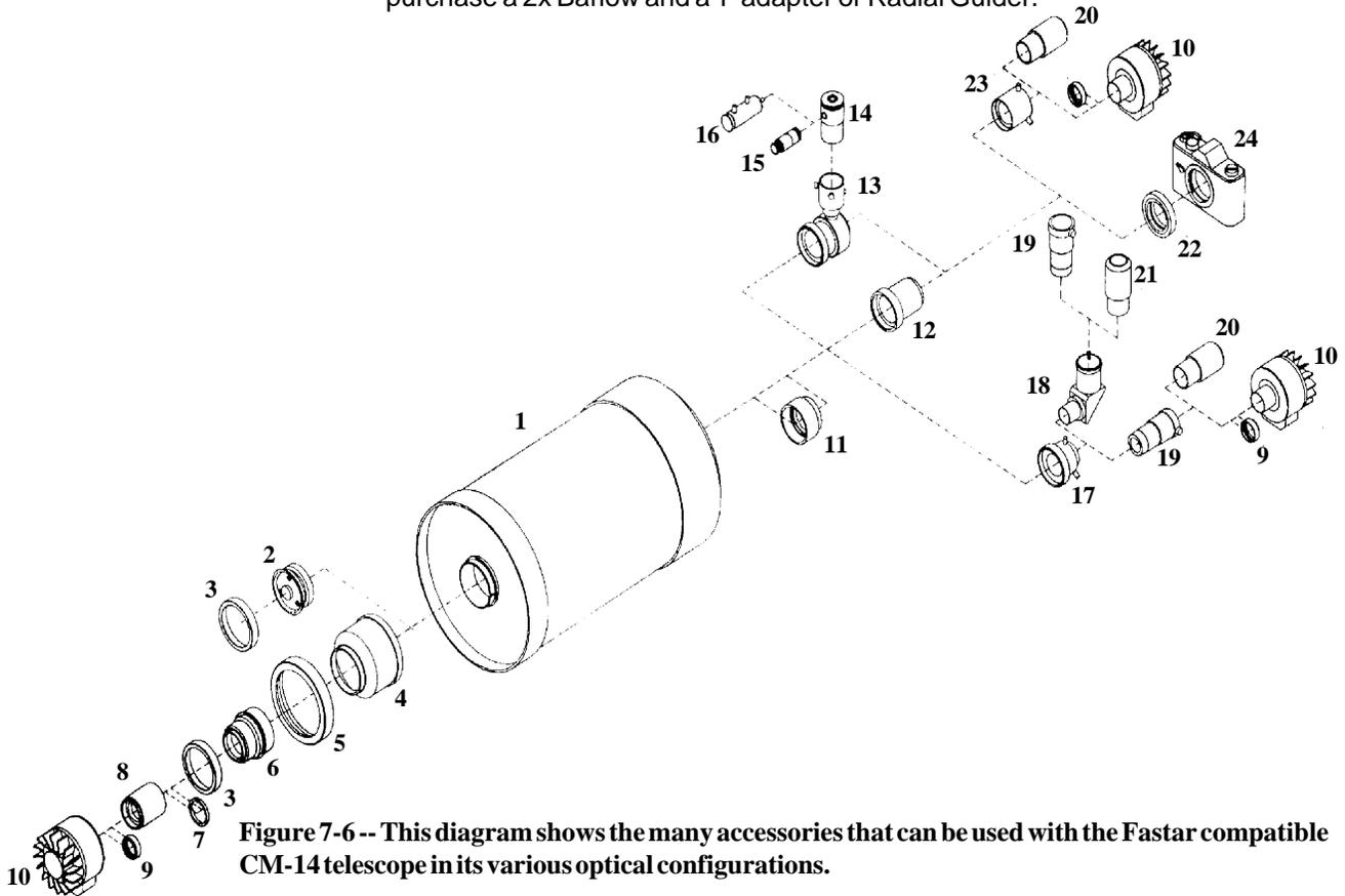
Figure 7-6-- This diagram shows the many accessories that can be used with the Fastar compatible CM-14 telescope in its various optical configurations.
