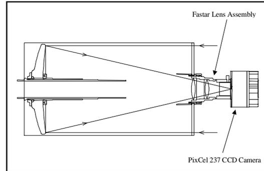
Figure 7-3 -- Light path at Fastar f/2.1 focus
