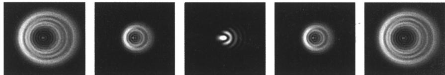
**Figure 8-1 -- Even though the star pattern appears the same on both sides of focus, they are asymmetric. The dark obstruction is skewed off to the left side of the diffraction pattern indicating poor collimation.**
