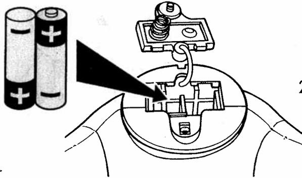
2. Take out the old batteries, replace with 2 "AAA" alkaline batteries (not included) as shown. Replace door.
