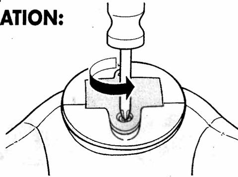
1. Using Phillips head screwdriver (not included), unscrew door and remove.
