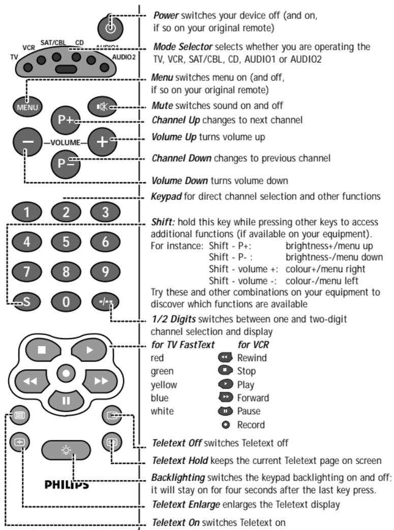
**Try it out!** The easiest way to find out how your new remote works, is to try pressing the keys and see what happens - don't worry, you won't damage anything! Most of the keys work just like on your original remote control. Of course, if your TV or VCR does not offer a specific function, pressing that key will have no effect.
