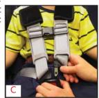
**6** Position the harness straps around the child and fasten the child restraint buckle (*Fig. C*). Proper connection is confirmed with a positive click after inserting the second buckle tongue.
