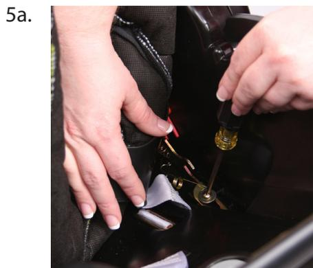
Place the assembled spring into the screw hole.
