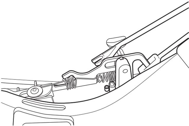
Spring should be attached to metal bracket as shown below.
