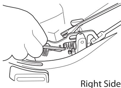
Using the slotted end of wrench provided, push hook and insert directly above current spring onto metal bracket as shown in figure 6b.
