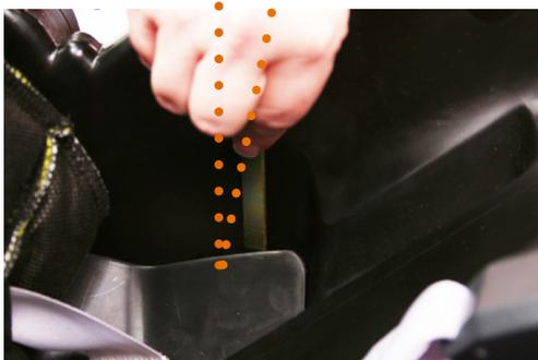
Slide wrench tool underneath lower end of plastic cover to pop open.
