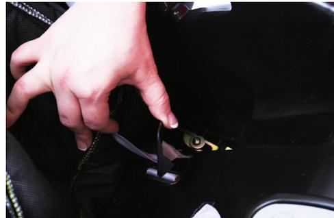
While holding back plastic cover, use Phillips-head screwdriver to remove screw and washer as shown in figure 3b.
