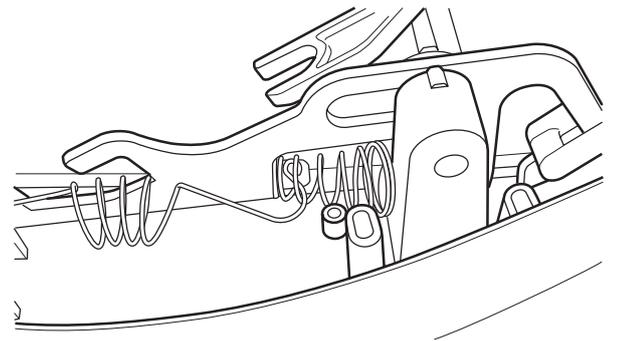
Spring should NOT be attached to permanent spring as shown below.
