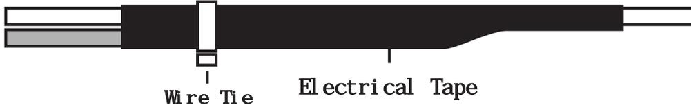
CAUTION: All wires must be wrapped with tape and wire tied.
