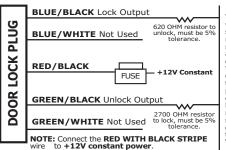
wire door locking system and will require two (2) resistors to lock and unlock the doors. Locate the WHITE/DK WHITE/DK GREEN wire in the driver's kick panel. This wire controls the door locks. Add the resistors as stated in the stated in the diagram, Wire the unit in as a Type A" system.
