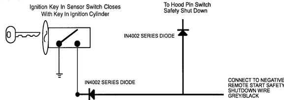
**Note:** A second 4002 series diode may be required to maintain the integrity of the hood open, shut down circuit. If this is the case, it must be installed as shown in the diagram above. The anode (Non Striped) side must be connected to the Gray/Black wire of the Remote Start Unit. The cathode (Striped) side must be connected to the hood pin switch. If the hood pin switch is also used for an alarm trigger input, be certain to use the dual diode set up shown earlier in this manual.
