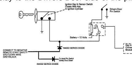
**Note:** A second 4002 series diode may be required to maintain the integrity of the hood open, shut down circuit. If this is the case, it must be installed as shown in the diagram above. The anode (Non Striped) side must be connected to the Gray/Black wire of the Remote Start Unit. The cathode (Striped) side must be connected to the hood pin switch. If the hood pin switch is also used for an alarm trigger input, be certain to use the dual diode set up shown earlier in this manual.
