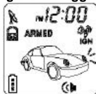
**CLEAR THE FLASH ICON AND MELODY SOUND:** While triggering the alarm the LCD screen will alert user through melody sound and flashing trigger icon, press the **SET** button 3 times within 3 seconds will clear the flash icon and stop melody sound on the LCD screen transmitter.
