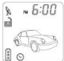
parking light will flash (6) times. The siren chirps (6) times. The vehicle is now programmed to start at the real time of the next day. Your set time for the next day engine start flashes for approx. 3 seconds on the LCD screen. After 3 seconds the 🕒 icon stays displayed on the LCD screen.
