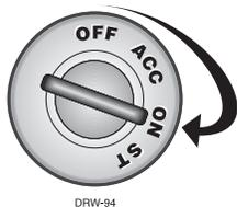
1. Insert the ignition key and turn it to the ON (not the START) position.
