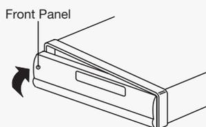
3. Note that if the front panel fails to lock in position properly, pressing control button may not function and the display may be missing some segments. Press the **OPEN/CLOSE** button and then reinstall the front panel again.
