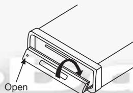
2. Press the **OPEN/CLOSE** button again, the front panel will slide up.
