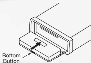
2. When the panel bracket is in slide-up position, insert one side of the front panel to its proper position and push the other side into the panel bracket, a 'click' sound should be heard.
