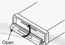
3. When the front panel slides down, press the bottom button of the front panel upward and pull it out from the panel bracket.
