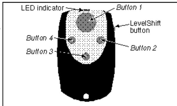
use the most — button 1 to arm, disarm, lock and unlock the doors — is larger than the others. Buttons 2, 3 and 4 are the smaller buttons to the right, below and left of button 1. The *LevelShift* button on the side lets you select channels 5–12:
