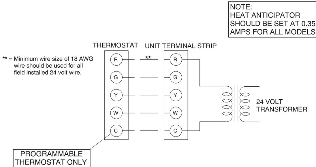
**FIGURE 3 - TYPICAL FIELD CONTROL WIRING DIAGRAM**
