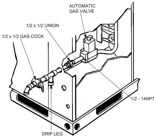
**FIGURE 5 - EXTERNAL SUPPLY CONNECTION
