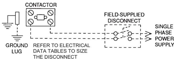
**FIGURE 4 - TYPICAL FIELD POWER WIRING DIAGRAM**
