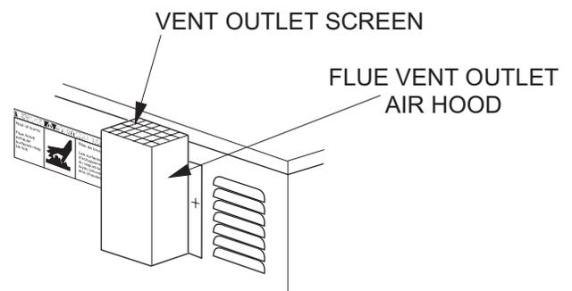
**FIGURE 6 - FLUE VENT OUTLET AIR HOOD**
