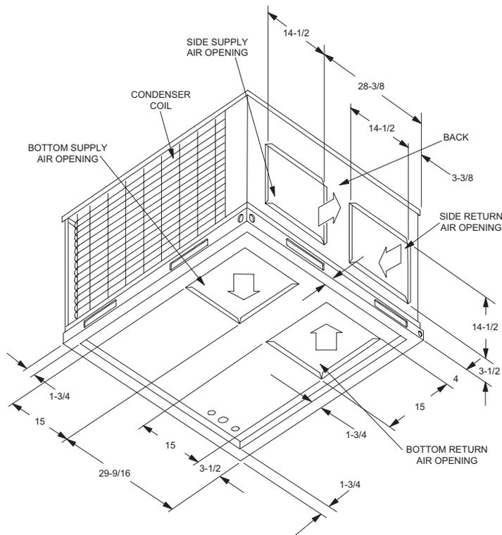
**FIGURE 9 - UNIT DIMENSIONS - BACK & BOTTOM**
