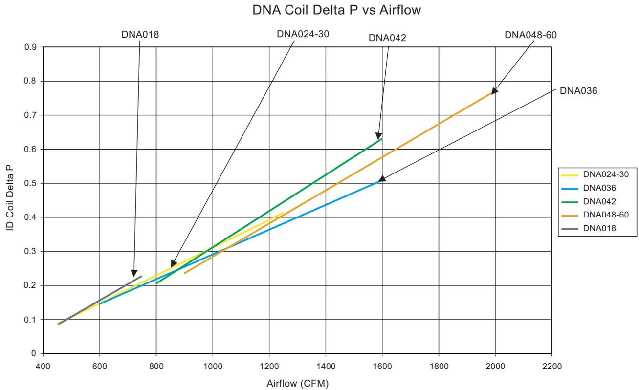
**FIGURE 13 - DNA COIL DELTA P VS. AIRFLOW**
