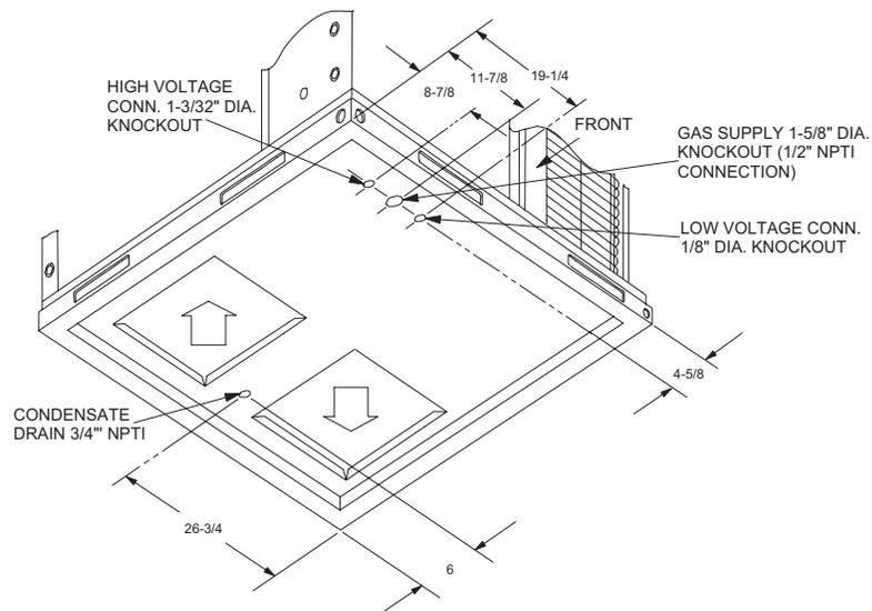
**FIGURE 8 - UNIT DIMENSIONS - FRONT & BOTTOM**
