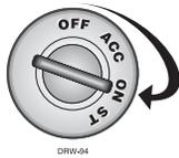
To disarm the security system, turn the ignition to the ON position. Press the override switch the preset number of times (one to five times) within 15 seconds. After five seconds the system will disarm. If the system does not disarm, you may have waited too long; turn the ignition off and on and try again.
