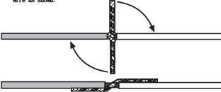
Use electrical tape to wrap, be sure to cover about 2 inches on either side of connection. Secure with wire ties as shown.
