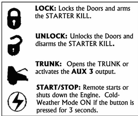
Note: Pressing the LOCK and UNLOCK buttons at the same time will activate the AUX 2 output.
