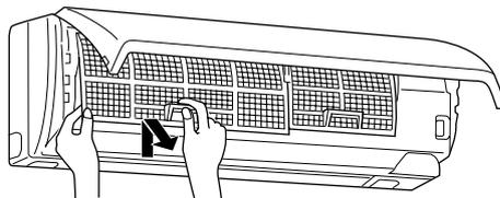
(2) Remove the air cleaning filter (Blue bellows type) from the catechin air filter.
