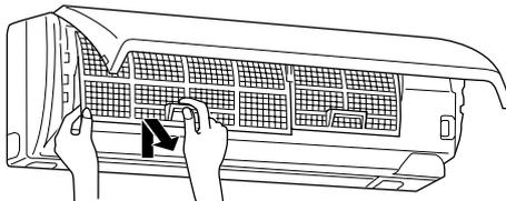
(2) Remove the air cleaning filter (Blue bellows type) from the catechin air filter.
