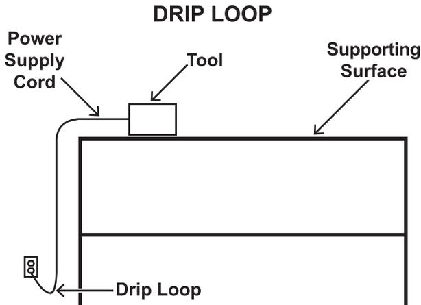
1. To avoid the possibility of the tool plug or receptacle getting wet, position tile saw to one side of a wall mounted receptacle to prevent water from dripping onto the receptacle or plug. The user should arrange a “drip loop” in the cord connecting the saw to a receptacle. The “drip loop” is that part of the cord below the level of the receptacle, or the connector if an extension cord is used, to prevent water traveling along the cord and coming in contact with the receptacle.
