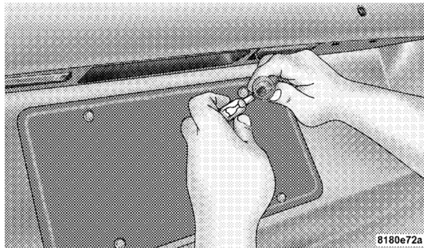
Removing Bulb From Socket
