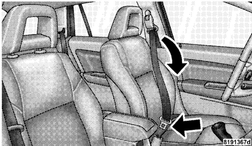
Inserting Latch Plate Into Buckle
