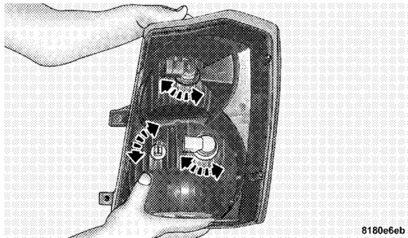
Removing Socket And Bulb
