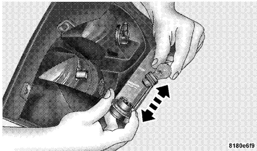
Removing Bulb From Socket
