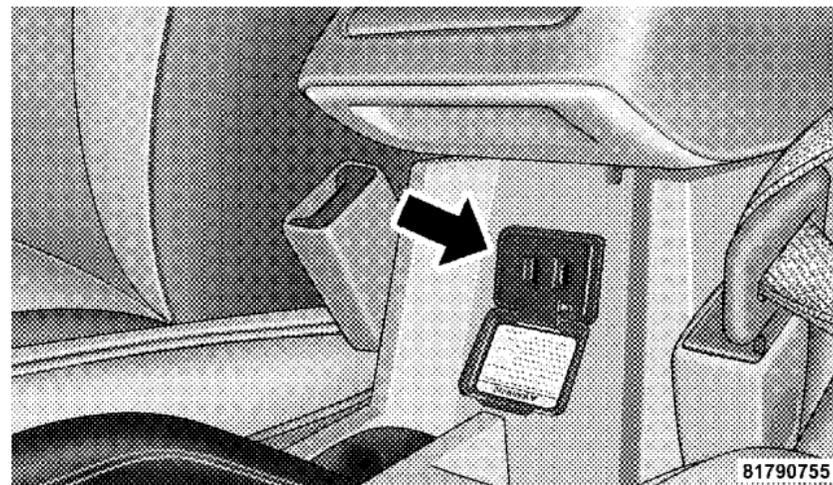
Power Outlet — 115 Volts (150 Watts)
