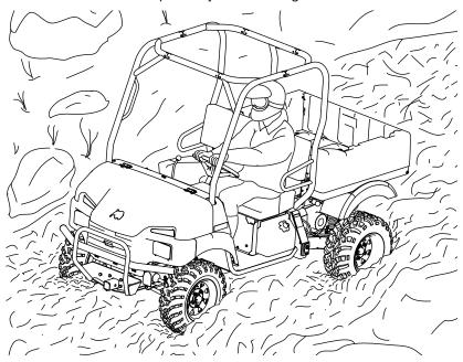
NOTE: After running your vehicle in water, it's critical that you perform the services outlined in the Maintenance section on page 47. Give special attention to engine oil, transmission oil, front and rear gearcases, and all grease fittings.
