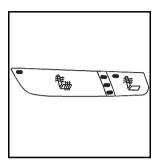
On vehicles with heated seats, the buttons are on the front doors. The ignition must be on to use this feature.
