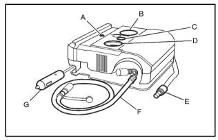
When using the tire sealant and compressor kit during cold temperatures, warm the kit in a heated environment for five minutes. This will help to inflate the tire faster.
