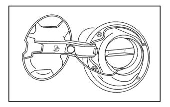
The tethered fuel cap is located behind a hinged fuel door on the driver side of the vehicle. If the vehicle has E85 fuel capability, the fuel cap will be yellow and state that E85 or gasoline can be used. See *Fuel E85* (85% Ethanol) on page 6-8.
