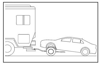
The vehicle can be towed using a dolly. To tow the vehicle using a dolly, follow these steps:
