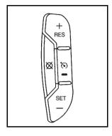
The cruise control buttons are located on the left side of the steering wheel.
