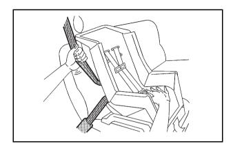
6. To tighten the belt, push down on the child restraint, pull the shoulder portion of the belt to tighten the lap portion of the belt, and feed the shoulder belt back into the retractor. When installing a forward-facing child restraint, it may be helpful to use your knee to push down on the child restraint as you tighten the belt.
