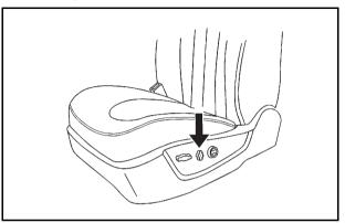
Use the vertical control on the outboard side of the seat to adjust the seatback.
