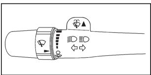
The windshield wiper lever is located on the left side of the steering column. Turn the band with the wiper symbol on it to control the windshield wipers.
