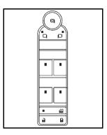
On vehicles with power windows, the switches are on the driver door armrest. Each passenger door has a switch that controls only that window.
