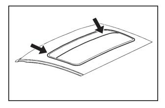
Dirt and debris may collect on the sunroof seal or in the tracks that could cause an issue with sunroof operation, noise or plug the water drainage system. Periodically open the sunroof and remove any obstacles or loose debris. Wipe the sunroof seal and roof sealing area using a clean cloth, mild soap, and water. Do not remove grease from sunroof.
