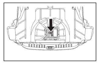
3. Turn the retainer clockwise and remove the tire sealant and compressor kit.
