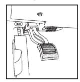
The parking brake pedal is located to the left of the regular brake pedal, near the driver door.
