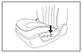
Use the round control on the outboard side of the seat to adjust the lumbar support.
