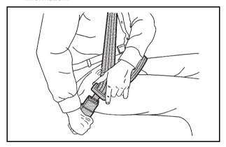
Push the latch plate into the buckle until it clicks.If the latch plate will not go fully into the buckle, check if the correct buckle is being used. Pull up on the latch plate to make sure it is secure. If the belt is not long enough, see *Safety Belt Extender on page 2-31*.
