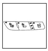
On vehicles with heated and ventilated seats, the buttons are on the front doors. The ignition must be on to use this feature.
