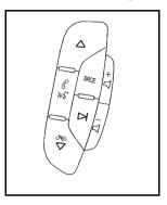
Vehicles with audio steering wheel controls could differ depending on the vehicle's options. Some audio controls can be adjusted at the steering wheel.
