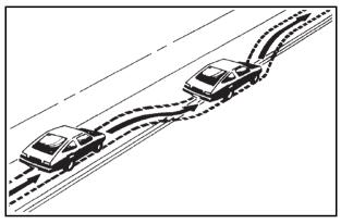
If the level of the shoulder is only slightly below the pavement, recovery should be fairly easy. Ease off the accelerator and then, if there is nothing in the way, steer so that the vehicle straddles the edge of the pavement. Turn the steering wheel 8 to 13 cm (3 to 5 inches), about one-eighth turn, until the right front tire contacts the pavement edge. Then turn the steering wheel to go straight down the roadway.
