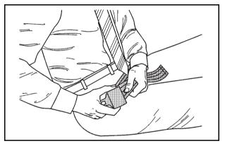
To make the belt longer, tilt the latch plate and pull it along the belt.
