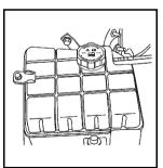
Fill the coolant surge tank with the proper mixture to the FULL COLD mark on the side of the coolant surge tank.
