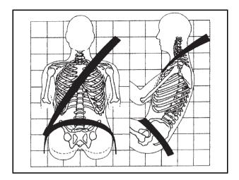
Sit up straight and always keep your feet on the floor in front of you. The lap part of the belt should be worn low and snug on the hips, just touching the thighs. In a crash, this applies force to the strong pelvic bones and you would be less likely to slide under the lap belt.
