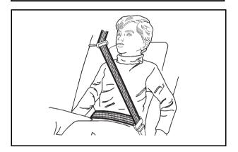
4. Buckle, position, and release the safety belt as described previously in this section. Make sure the shoulder portion of the belt is on the shoulder and not falling off of it. The belt should be close to, but not contacting, the neck.
