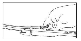
4. Replace the blade assembly with a new one.
