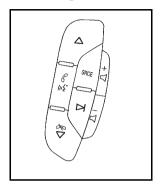
For vehicles with audio steering wheel controls, some audio controls can be adjusted at the steering wheel.
