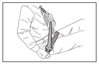
To make the lap part tight, pull up on the shoulder belt. It may be necessary to pull stitching on the safety belt through the latch plate to fully tighten the lap belt on smaller occupants.
