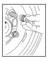
8. Remove all wheel nuts and remove the flat tire.
