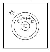
The exterior lamp control is located on the instrument panel to the left of the steering wheel.
