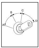
In order to shift out of P (Park), ignition must be in the ON/RUN and the regular brake pedal must be applied.
