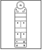
The power window switches are located on the driver's door armrest. In addition, each door has a switch for its own window.
