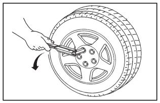
2. Turn the wheel wrench counterclockwise to loosen all the wheel nuts, but do not remove them yet.
