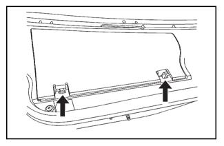
Insert a tool behind the push pin located on the inboard side of the air filter compartment to carefully pry the pin out.
