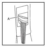
Press the release button (A) and move the height adjuster to the desired position. The adjuster can be moved up by pushing up on the shoulder belt guide.
