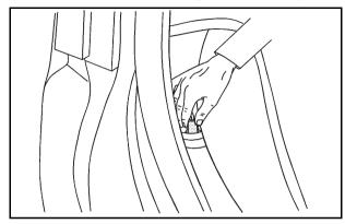
Remove the guide from its storage pocket on the rear side of the seatback.
