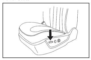
Use the horizontal control on the outboard side of the seat to adjust the seat.
