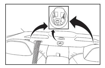
The top tether anchors are located under the covers on the rear seatback filler panel. Flip open the cover to access the anchors. Be sure to use an anchor located on the same side of the vehicle as the seating position where the child restraint will be placed.
