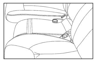
The vehicle may have a front center seat. This seat can be converted to a storage area by lowering the seatback. See *Center Flex Storage Unit on page 3-47*.
