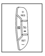
The cruise control buttons are located on left side of the steering wheel.
