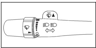
The windshield wiper lever is located on the left side of the steering column.
