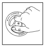
2. Turn the center retainer counterclockwise to remove it.
