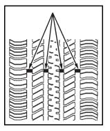
One way to tell when it is time for new tires is to check the treadwear indicators, which will appear when your tires have only 1/16 inch (1.6 mm) or less of tread remaining. See *Tire Inspection and Rotation on page 6-69* for additional information.
