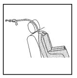
If the position you are using has a fixed headrest or head restraint and you are using a single tether, route the tether over the headrest or head restraint.
