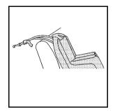
If the position you are using does not have a headrest or head restraint and you are using a dual tether, route the tether over the seatback.
