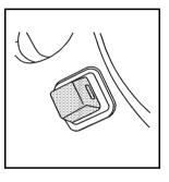
For vehicles with a power tilt control, it is located on the left hand side of the steering column.
