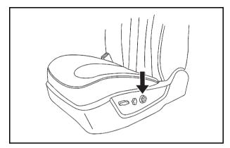
On vehicles with power lumbar, the control is on the outboard side of the seat.
