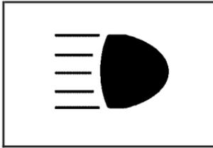
While the high beams are on, this light located on the instrument panel cluster will also be on.
