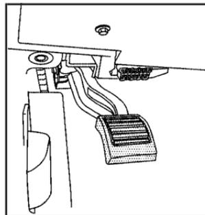
The parking brake pedal is located to the left of the regular brake pedal, near the driver door.
