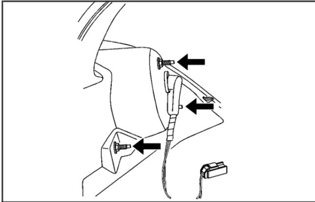
5. Remove the three hex nuts holding the taillamp assembly in place.
