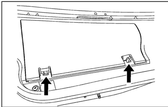
2. Insert a tool behind the push pin located on the inboard side of the air filter compartment to carefully pry the pin out.
