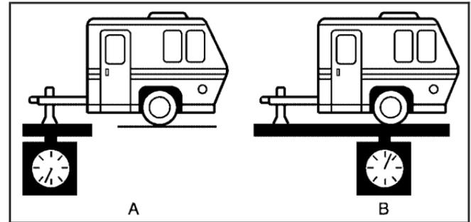
Using a weight-carrying hitch, the trailer tongue (A) should weigh 10 to 15 percent of the total loaded trailer weight (B).
