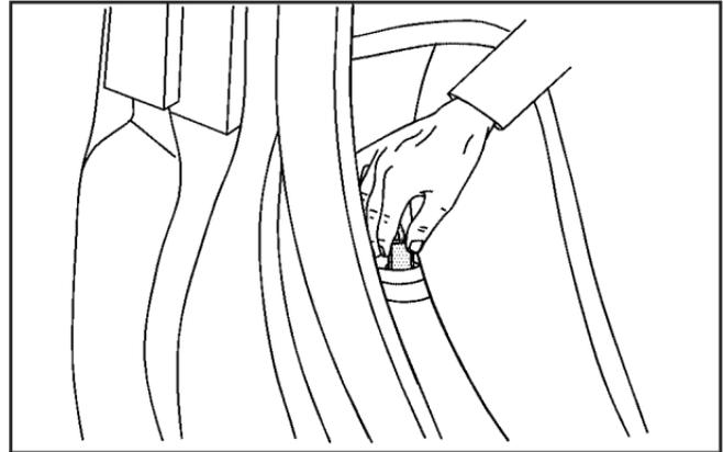
1. Remove the guide from its storage pocket on the rear side of the seatback.
