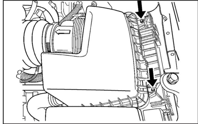
1. Remove the two screws on the top of the engine air cleaner/filter cover.
