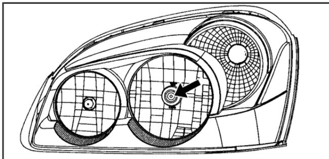
2. Locate the aim dot on the lens of the low-beam headlamp.
