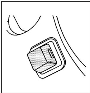
For vehicles with this feature, the power tilt wheel control is located on the left side of the steering column.
