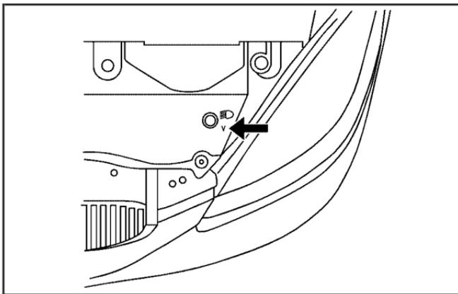
7. Locate the vertical headlamp aiming screws, which are under the hood near each headlamp assembly. The adjustment screw can be turned with a 6 mm male hex.
