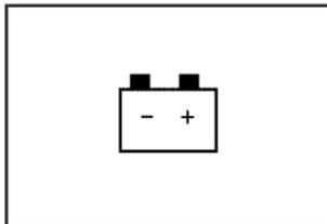
This light comes on briefly when the ignition key is turned to START, but the engine is not running, as a check to show it is working.
