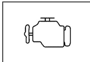
This light should come on when the ignition is on, but the engine is not running, as a check to show it working. If it does not, have the vehicle serviced by your dealer/retailer.
