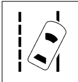
For vehicles with the lane departure warning system, this light briefly comes on green, while starting the vehicle, to indicate that it is working.
