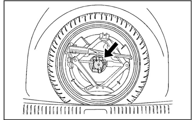
3. Lift and remove the compact spare tire cover.
