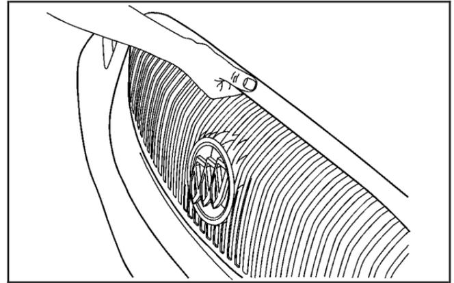
2. Then go to the front of the vehicle and pull the secondary hood release to the right. The hood latch is located under the hood, near the center, at the front edge of the grille.
