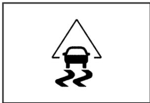
For vehicles with a Traction Control System (TCS) and StabiliTrak<sup>®</sup> warning light, this light comes on briefly when the engine is started.
