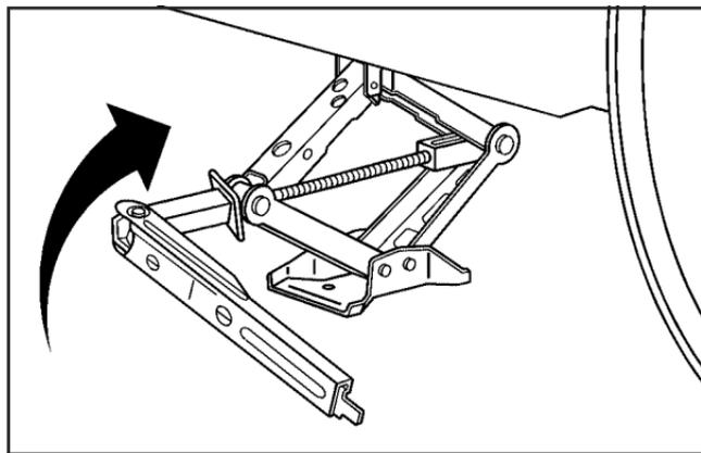
7. Turn the jack handle clockwise to raise the vehicle. Raise the vehicle far enough off the ground for the compact spare tire to fit under the vehicle.
