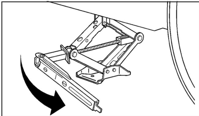
12. Lower the vehicle by turning the jack handle counterclockwise. Lower the jack completely.
