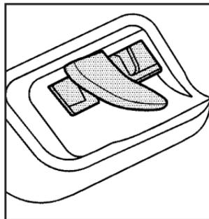
The tilt lever is located on the left side of the steering column.
