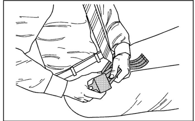
To make the belt longer, tilt the latch plate and pull it along the belt.
