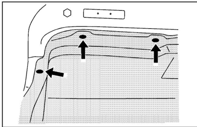
2. Remove the three fasteners from the trunk trim.
