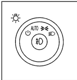
The exterior lamps control is located on the instrument panel to the left of the steering wheel.
