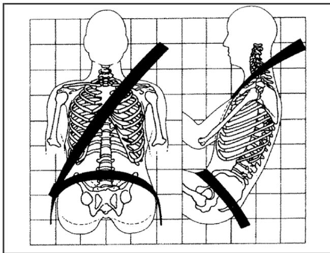
Sit up straight and always keep your feet on the floor in front of you. The lap part of the belt should be worn low and snug on the hips, just touching the thighs.
