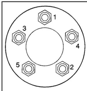
13. Tighten the wheel nuts firmly in a crisscross sequence as shown.
