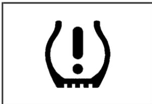
When a low tire pressure condition is detected, the TPMS illuminates the low tire pressure warning light located on the instrument panel cluster.
