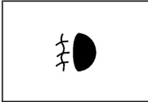
The fog lamp light comes on when the fog lamps are in use.
