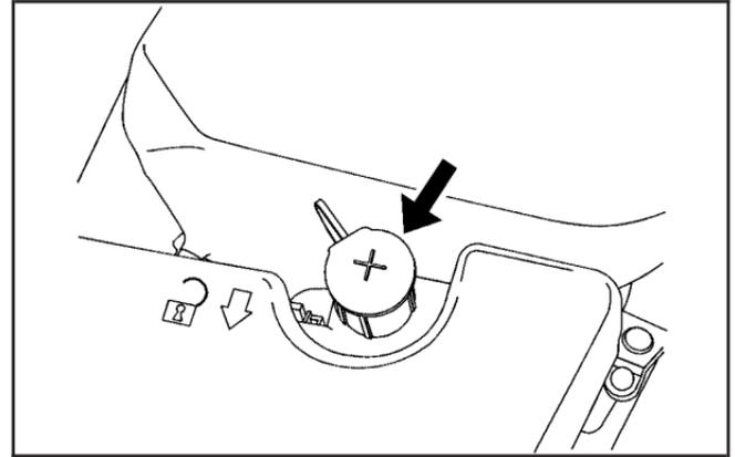
Access the remote positive (+) terminal by removing the cover.
