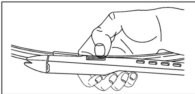
3. Squeeze the tabs on each side of the wiper blade assembly and slide the assembly off the end of the wiper arm.
