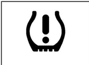
For vehicles with a tire pressure light, this light comes on briefly when the engine is started and provides information about tire pressures and the Tire Pressure Monitoring System.
