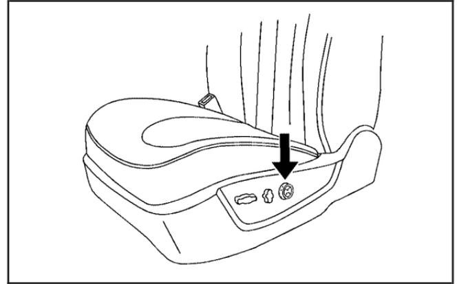
On vehicles with power lumbar, the control is located on the outboard side of the front seats.
