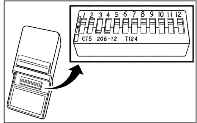
1. To verify that the garage door opener is a Fixed Code unit, remove the battery cover on the hand held transmitter supplied by the manufacturer of the garage door opener motor. If there are a row of dip switches similar to the graphic above, the garage door opener is a Fixed Code unit. If you do not see a row of dip switches, return to the previous section for Programming Universal Home Remote – Rolling Code.
