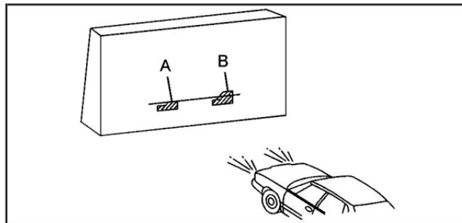
9. Make sure that the light from the headlamp is positioned at the bottom edge of the horizontal tape line. The lamp on the left (A) shows the correct headlamp aim. The lamp on the right (B) shows the incorrect headlamp aim.
