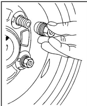
8. Remove all wheel nuts and remove the flat tire.
