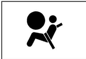
The airbag readiness light flashes for a few seconds when the engine is started. If the light does not come on then, have it fixed immediately.
