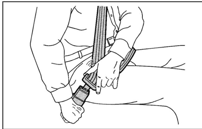
3. Push the latch plate into the buckle until it clicks. If the latch plate will not go fully into the buckle, check if the correct buckle is being used. Pull up on the latch plate to make sure it is secure. If the belt is not long enough, see *Safety Belt Extender* on page 1-34. Position the release button on the buckle so that the safety belt could be quickly unbuckled if necessary.
