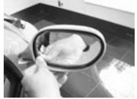
Side view mirrors are adjusted by pressing gently on the bottom corners of the right and left side of the mirror itself. Have someone help you set the passenger's side mirror for optimal rear view. You may install a blind spot mirror on the side mirror to give you a better peripheral view. These can be purchased at any auto parts store.
