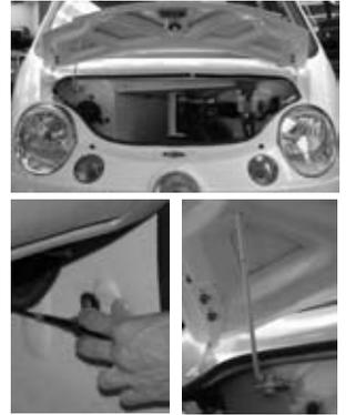
Inside the front deck lid you will find the brake fluid reservoir, the horn, and the windshield fluid tank. In the center you will see the access to the front tire and suspension. It is not recommended that you make any adjustments to braking or suspension systems aside from checking brake and windshield fluids regularly.
