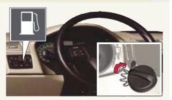
Press the button to open the fuel filler flap. Hang up the fuel filler cap during refuelling.
