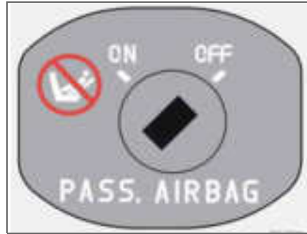
Switch for SRS in OFF position.
