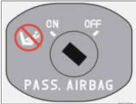
Switch for SRS in ON position.
