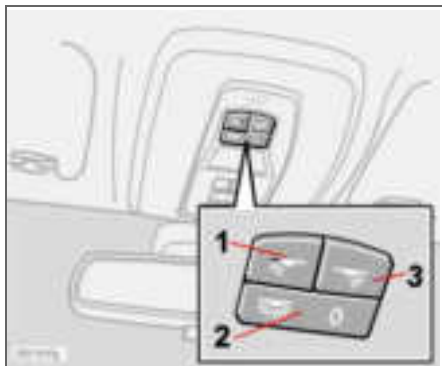
Passenger compartment lighting and reading lamps.
