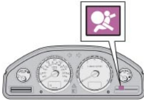
**Safety system warning light in the instrument panel**
