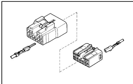
(b) Push the terminal retainer in to the full lock position.
