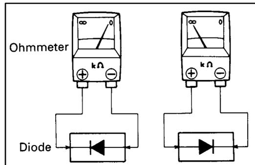
If the circuit has diodes, reverse the two leads and check again.
