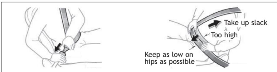
If belt is fully extended, then retracted even slightly, it cannot be re-extended beyond that point, unless fully retracted again. This feature is used to help hold child restraint systems securely.
