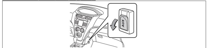
By inserting a mini plug of a commercially available component into the AUX audio jack, you can listen to music from a portable audio device through the vehicle’s speaker system while in AUX mode.
