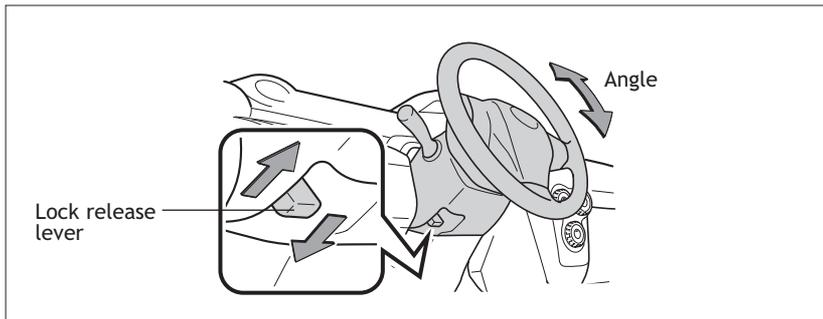
Hold wheel, push lever down, set angle and return lever.
