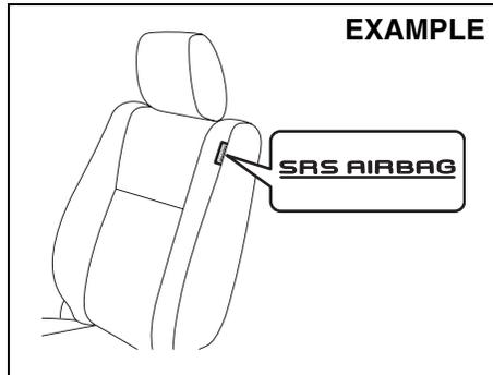
Side air bags are located in the part of the front seatbacks closest to the doors. The words "SRS AIRBAG" are indicated on the tag to identify the location of the side air bags.
