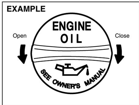
Remove the oil filler cap and pour oil slowly through the filler hole to bring the oil level to the upper limit on the dipstick. Be careful not to overfill. Too much oil is almost as bad as too little oil. After refilling, start the engine and allow it to idle for about a minute. Stop the engine, wait about 5 minutes and check the oil level again.
