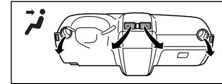
Temperature-controlled air comes out of the center and side air outlets.
