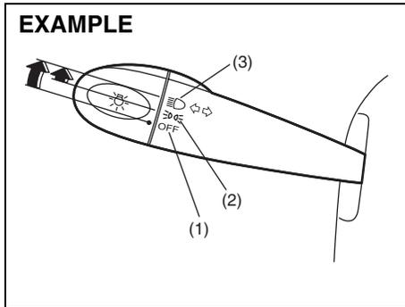
To turn the lights on or off, twist the knob on the end of the lever. There are three positions:
