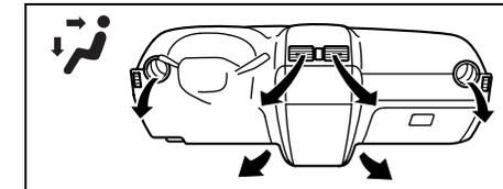
Temperature-controlled air comes out of the floor outlets and cooler air comes out of the center and side outlets. When the temperature selector (1) is in the fully COLD position or fully HOT position, however, the air from the floor outlets and the air from the center and side outlets will be the same temperature.
