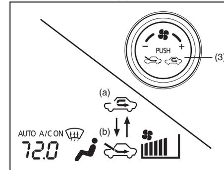
Push the air intake selector (3) to change between the following modes.
