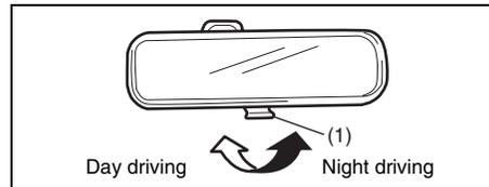
You can adjust the inside rearview mirror by hand so as to see the rear of your vehicle in the mirror. To adjust the mirror, set the selector tab (1) to the day position, then move the mirror up, down or sideways by hand to obtain the best view.
