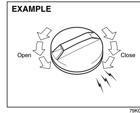
To remove the fuel filler cap:
