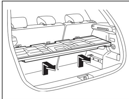
2) Lift the board, and remove the board from the vehicle.
