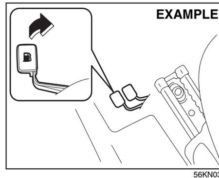
The fuel filler cap is located on the left rear side of the vehicle. The fuel filler door can be unlocked by pulling up the opener lever located on the outboard side of the driver's seat and can be locked by simply closing the door.
