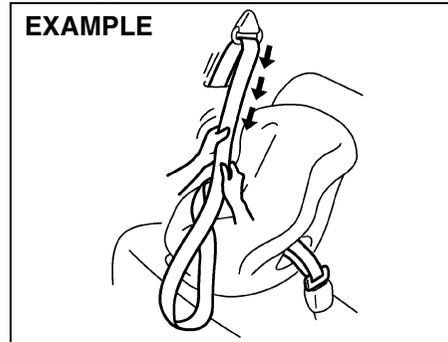
1) Pull all of the remaining webbing out of the retractor. You will hear a click, which means that the emergency locking retractor (ELR) has converted to function as an automatic locking retractor (ALR).
