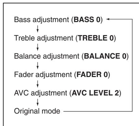
2) Turn the tone/balance/fader control knob (2) to adjust the sound.
