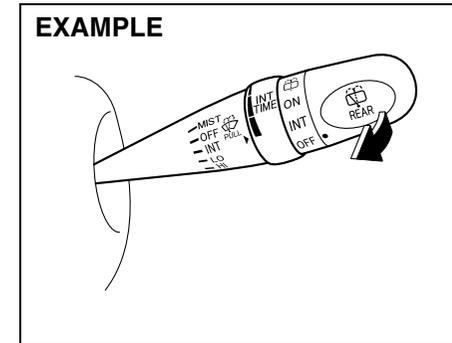
To spray windshield washer fluid, pull the lever toward you. The windshield wipers will automatically turn on at low speed if they are not already on and the “INT” position is equipped.
