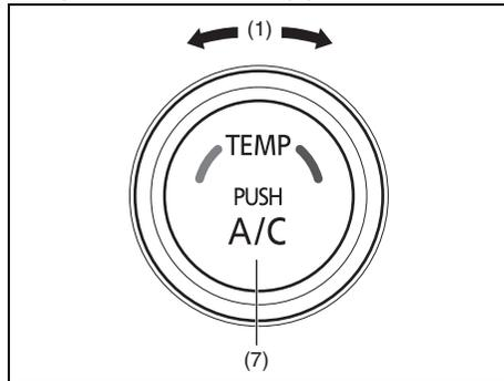
Turn the temperature selector (1) to adjust the temperature.
