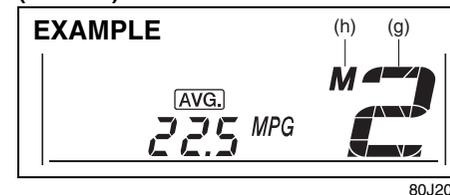
When the ignition switch is in the "ON" position, the display (C) indicates the gear position (g).
