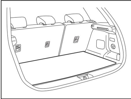
Your vehicle is equipped with the luggage compartment board in the luggage compartment. You can place luggage or other cargos on the board or under the board. You can also place tall luggage by stowing the board on the floor of the luggage compartment.
