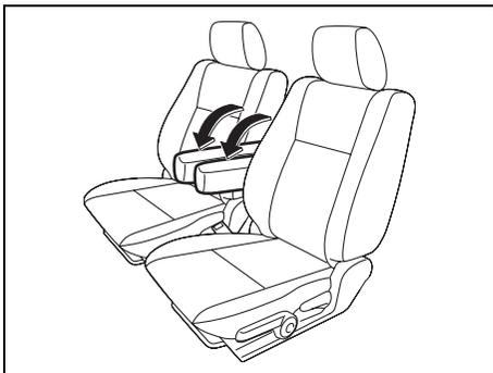
To use the armrest, pivot it down from the stowed (fully up) position. When not in use, return the armrest to the stowed position.
