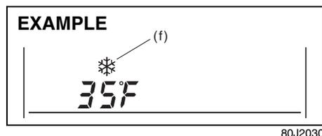
If the outside temperature nears freezing, the mark (f) will appear on the display.
