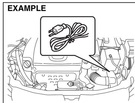
The engine block heater will help you start the engine more easily in very cold weather ( $-18^{\circ}\text{C}$  ( $0^{\circ}\text{F}$ ) or below). To use the engine block heater:
