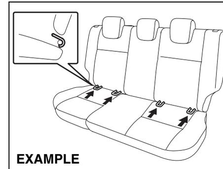
Your vehicle is equipped with lower anchors for securing up to one or two standard LATCH-type child restraint(s) in the rear seats. (LATCH stands for Lower Anchors and Tethers for Children.) The anchors are located where the rear of the seat cushion meets the bottom of the seatback.
