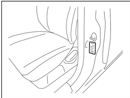
The front and rear tire pressure specifications for your vehicle are shown below and are listed on the Tire and Loading Information Label, which is located on the driver’s door lock pillar. The Tire and Loading Information Label contains the following information:
