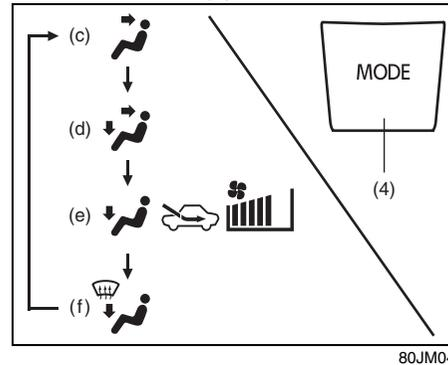
Push the air flow selector (4) to change among the following functions. The indication of the selected mode appears on the display.
