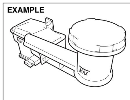
Check the brake fluid level by looking at the reservoir in the engine compartment. Check that the fluid level is between the "MAX" and "MIN" lines. If the brake fluid level is near the "MIN" line, fill it up to the "MAX" line with SAE J1703 or DOT3 brake fluid.
