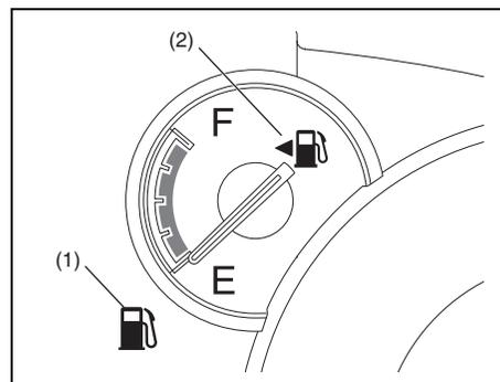
When the ignition switch is in the "ON" position, this gauge gives an approximate indication of the amount of fuel in the fuel tank. "F" stands for full and "E" stands for empty.
