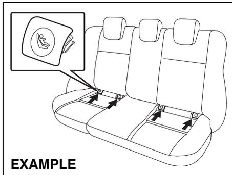
For SX4 SEDAN, the covers marked with the child restraint symbol as shown in the illustration indicate the presence of lower anchors. Remove the covers before installing the child restraint system. Cover the lower anchors when not in use.
