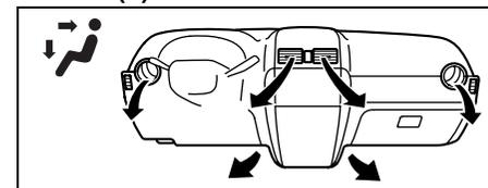
Temperature-controlled air comes out of the floor outlets and cooler air comes out of the center and side outlets. When the temperature selector (1) is in the fully COLD position or fully HOT position, however, the air from the floor outlets and the air from the center and side outlets will be the same temperature.
