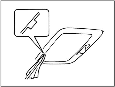
Pull down the lens by using a flat blade screwdriver covered with a soft cloth as shown. To install it, simply push it back in.
