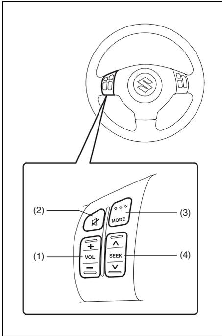
You can control basic functions of the audio system with the switches on the steering wheel.
