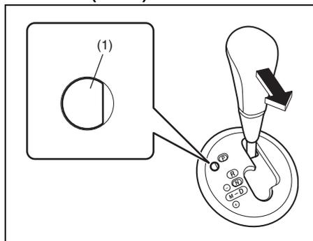
Vehicles with a CVT have an electrically operated park-lock feature. If the vehicle's battery is discharged, or there is some other electrical failure, the CVT cannot be shifted out of Park in the normal way. Jump starting may correct the condition. If not, follow the procedure described below. This procedure will permit changing the transaxle out of Park.
