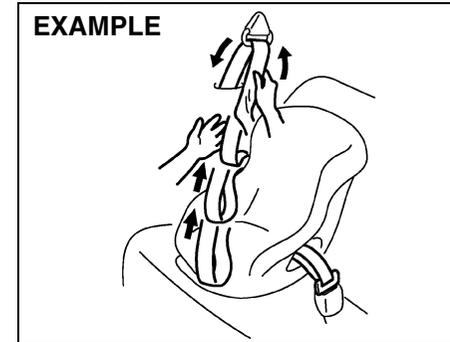
2) Allow the extra webbing to retract, and pull the webbing toward the retractor to take up any slack. Make sure that the lap portion of the belt is tight around the child restraint system and the shoulder portion of the belt is positioned so that it cannot interfere with the child's head or neck.
