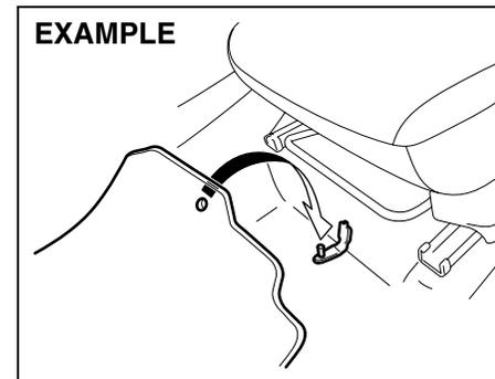
Your vehicle has a fastener to keep the driver's side floor mat from sliding forward and possibly interfering with the pedals. Whenever you put the driver's side floor mat back in the vehicle after it has been removed, be sure to hook the floor mat grommet(s) to the fastener(s) and position the floor mat properly in the footwell.
