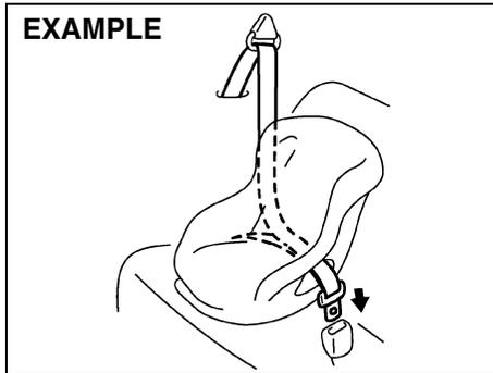
Install your child restraint system according to the instructions provided by the child restraint system manufacturer. If you install the child restraint system in the front seat, be sure to slide the seat to the rearmost position. After making sure that the seat belt is securely latched:
